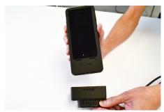
Align the charging contacts on the CT3043 case with those on the charge head.
