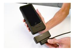
Once the devices are fully charged, pull the Charge Cup from the CT3043 case.
