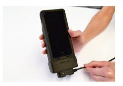
Place the case into the Charge Cup to charge.
