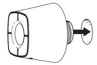
Below fixture: Fully tighten plastic nut onto puck behind wall.
