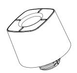
Drill a 29 mm (1.125") hole in fixture. Wipe fixture with alcohol wipe provided. Let it dry completely.
