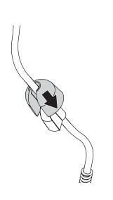
Firmly plug sensor cable into plastic nut assembly and pull on cable to confirm it is locked in.
