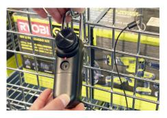
Place a charged and coded OneKEY against the lens on the lock and press the button the Key. The LED on the Key and the lock will flash green.
