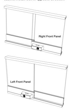
Make sure lock is unlocked using IR2 Key. Slide Plunger Lock through hole in front panel.
