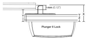
Note: If "Y" is greater than 20.5 mm (0.81") but less than 24.5 mm (0.96"), then plunger extension is required. Attach extension when plunger is extended using small screw provided.
