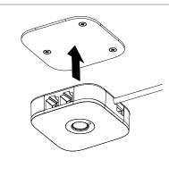
If routing the power cable through fixture, drill a 19mm hole minimum in fixture and direct the power cable straight down through the hole. Clean the surface of any dust or debris caused during drilling using the provided wipe and press alarm unit firmly against the surface for at least 10 seconds.
