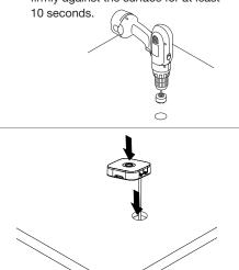
For all mounting methods, be sure the plunger switch on the bottom of the alarm unit is engaged with the surface.
