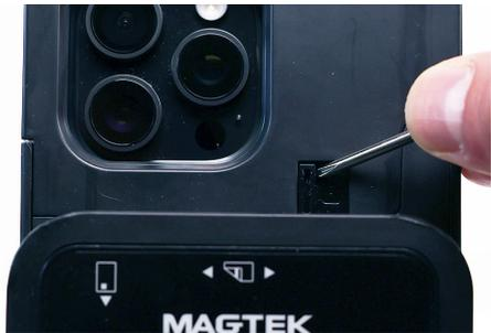
**17** Slide the locking tab to the left so that the lock icon is fully visible.
