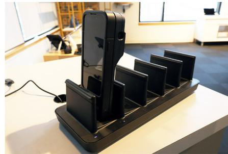
**18a** The cases can be charged using the gang charger. The LED next to the bay on the charger where the cases are placed will blink to indicate charging. Both devices will be charged when connected.
