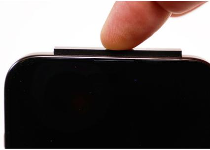
**14c** Center the spacer onto the top of the iPhone 15 Pro Max and apply pressure for at least 10 seconds.
