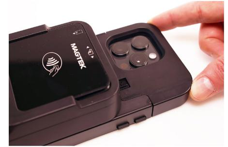
**16** Slide the DynaFlex II Go case down to expose the locking tab. Replace the cover onto the iPhone case.
