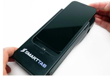
**15** Slide the iPhone into the case. Ensure that the USB-C connector plugs into the port on the iPhone.
