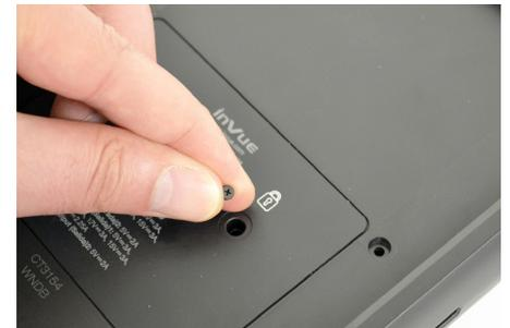
**66a Optional:** To lock the payment device case to the host case, first ensure that the screw holes are aligned. Then insert the 2 small screws.
