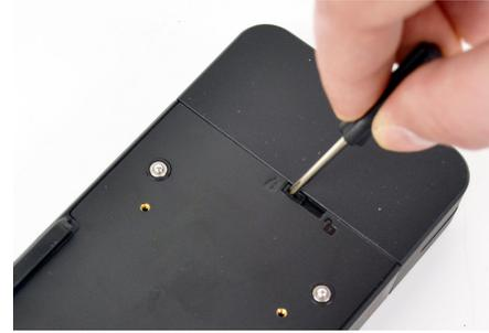
27 Slide the locking tab to the locked position.
