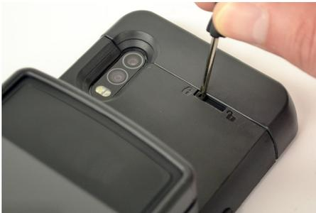
**52** Slide the locking tab to the locked position.
