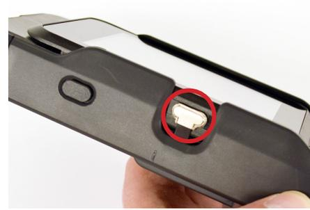
19 Plug the USB-C connector into the side of the payment device.
