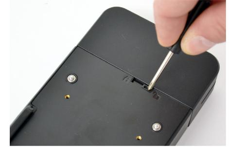
20 Slide the locking tab on the payment device case to the unlocked position using the provided small screwdriver.
