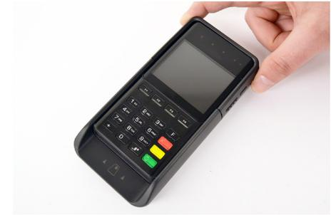
32 Replace the cover onto the case.
