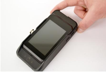
17 Replace the cover onto the case.
