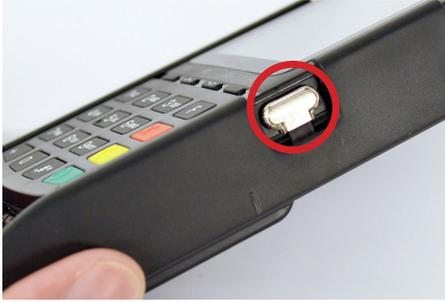
25 Plug the USB-C connector into the side of the payment device.
