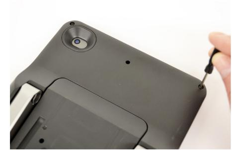
**74** Tighten the 2 screws (3 screws if using the CT3168 case).
