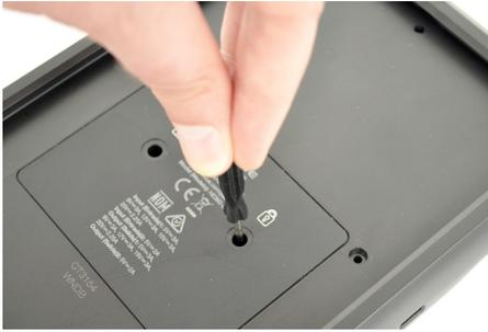
**66b** Tighten the 2 small screws using the small screwdriver.
