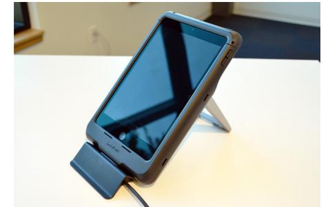
**76b** The tablet case can also be used with the single position charger (CT3051) mounted in the charger stand (CT3053). Deploy the kickstand and place the tablet case onto the charger.
