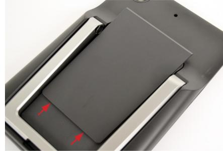
**62b** Slide the cover up from the bottom of the tablet case.
