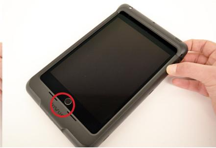
**72** Ensure that the tablet is fully inserted into the case and fully seated on the power connector.
