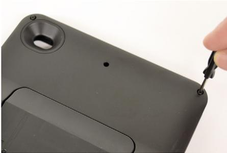
**68a** Use the small screwdriver to loosen the 2 screws in the top of the tablet case.
