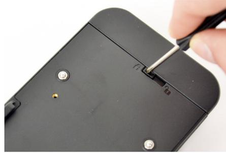
18 Slide the locking tab to the locked position.
