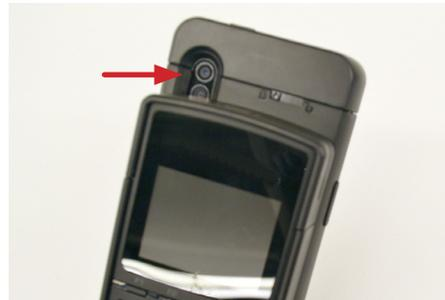
**53a** In the "home position", the camera on the host device may be blocked by the payment device case.
