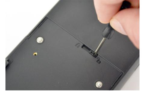
28 Slide the locking tab on the payment device case to the unlocked position using the provided small screwdriver.
