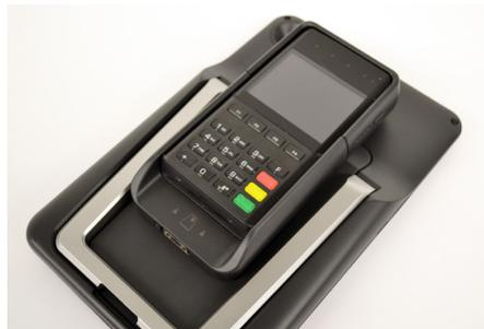
**64** Place the payment device case onto the host device case.
