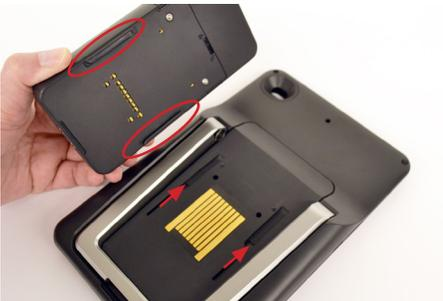
**63** To install a payment device case to a tablet host case, align the tabs on the payment device case with the slots on the host device case.
