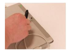
**REVOMAL**- place a DBG400 magnet key onto the back of the quick connect sensor. Slide the quick connect sensor out of the tablet sensor.
