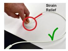
Make sure the strain relief on the anchor is facing AWAY from laptop. This will prevent the cable from getting caught under the laptop. Place the anchor behind the laptop and apply pressure for 10 seconds.
