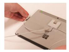
4 Plug the sensor into the tablet.
