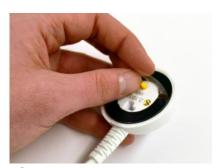
6 Peel the clear film from the adhesive on the anchor side of the unit.
