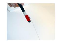
2 Slide the tether over the stylus as shown.
