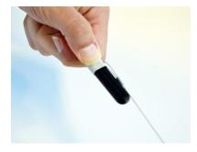
Press the tether against the 4 stylus for at least 10 seconds.
