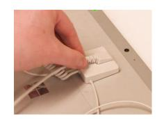
10 Slide the quick connect sensor (DKTR702-G) onto the tablet sensor, it will click into place.
