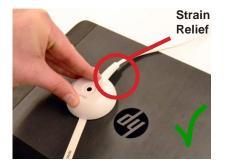
**5a** Place the alarm side onto the back of the laptop. Make sure the strain relief on the cable is clear of the laptop hinge. Apply pressure for 10 seconds.
