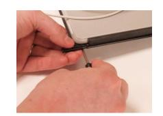
Insert the smaller provided screw onto the innermost hole on the bar. Use the small provided screwdriver to tighten the screw.
