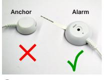
3 Select the side of the unit with the IR dot and labeled "alarm".
