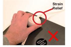
**5b** Do **NOT** place the strain relief near the laptop hinge.
