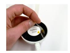
Peel the clear film from the adhesive on the alarm side of the unit.
