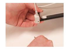
8 Place the keyboard sensor onto the bar. Make sure that the hole aligns with the one on the end of the bar.
