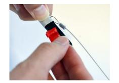
3 Pull the red tab from the tether to expose the adhesive.
