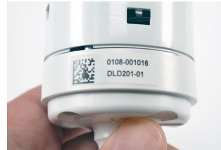
**3** Use the smart phone or tablet's camera to scan the barcode on the sensor (the Device ID can also be entered manually). Follow the prompts in the app to set up the sensor.
