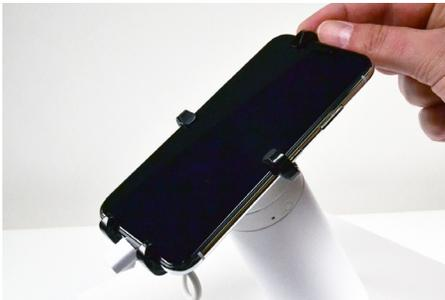
32 Hook the upper arm onto the device. It will automatically re-lock itself.
