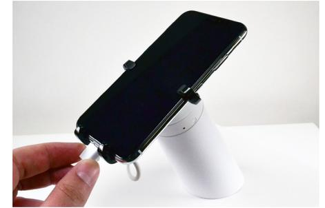
31 Plug the power connector back into the device.
