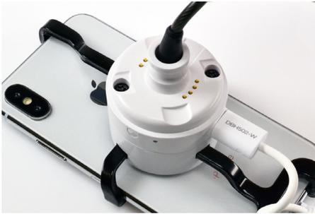
**20** Pull the sensor cable from a previously installed OnePOD stand and plug it into the sensor.
