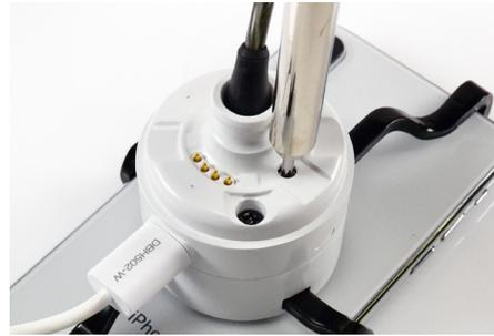
**21** **Optional:** If using a DLD211 sensor with the lock-out screw, use a TT8 bit to raise the screw to the sensor bit surface to lock the sensor to the sensor cable.
