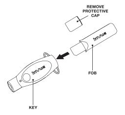
Confirm fob is flush with key. Press button of key to transfer security code. The green LED will blink twice when code has been correctly read.
