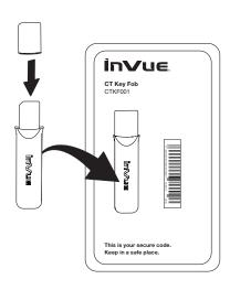
Place key against IR window of new InVue product. Press button to transfer secure code to product. The green LED will blink once to confirm a successful transfer.
