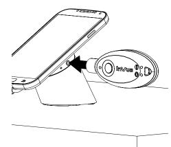
Remove the sensor and device from the stand. Place the magnet key (DBG400 or DBG406) into the depression on the sensor and push it inward to release the sensor cable. Pull the cable free.
