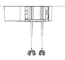
Use the scraper removal attachment (DNTX93) to break the adhesive bond between the stand and the surface. Use the scraper to remove the recoiler from beneath the fixture.
