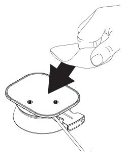
9 Remove the adhesive from its backing and place it on the puck. If there is a yellow plunger present on the puck, ensure that it fits into the cutout on the adhesive. Apply pressure for at least
