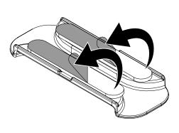
Pull the power connector cable gently across the back of the device to remove the slack and place the cable manager over the cable to hold it in place. Apply pressure for at least
