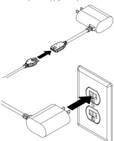
If using a USB-C device use the PS564 power supply. Plug the stand's power cable into the power supply. Connect the power cable to the power supply and plug it into a power outlet.
