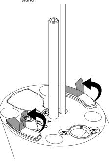
Route the power cable and stud down through a hole or slot in the fixture.
