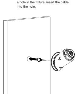
If routing the power cable through
