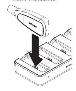
If using the Single Key Charger (OK4101), slide the OneKEY into the charger. Ensure that the charging contacts on the OneKEY align with the charging contacts on the charger.
