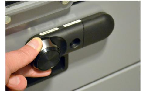
**27b** You will have several seconds to turn the knob to unlock and open. If the LED on the lock flashes red before the lock is opened, it will need to be unlocked again.
