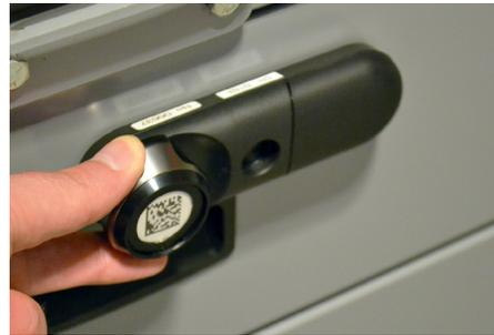
**30b** You will have several seconds to turn the knob to unlock and open. If the LED on the lock flashes red before the lock is opened, it will need to be unlocked again.
