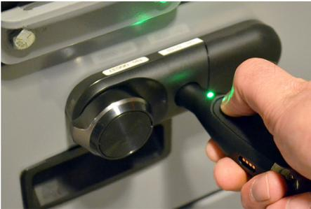
**26a** **Lock Activation Using OneKEY:** Place a charged and coded OneKEY against the lens on the lock and press the button the Key. The LED on the Key and the lock will flash green.
