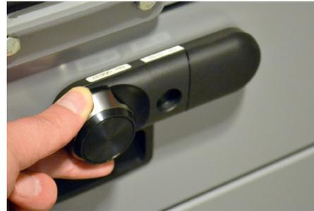
**26b** You will have several seconds to turn the knob to unlock and open. If the LED on the lock flashes red before the lock is opened, it will need to be unlocked again.
