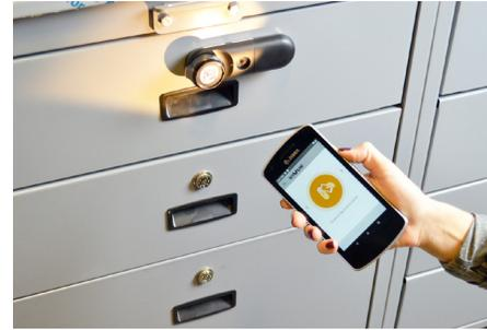
**29a Lock Activation Using Scanning Device:** If your smart device has a built in barcode reader, aim and scan the code on the front of the lock while the InVue LIVE Access App is open. Once confirmed by the App displaying “unlocked” and the LED flashing.
