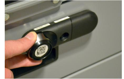
**29b** You will have several seconds to turn the knob to unlock and open. If the LED on the lock flashes red before the lock is opened, it will need to be unlocked again.
