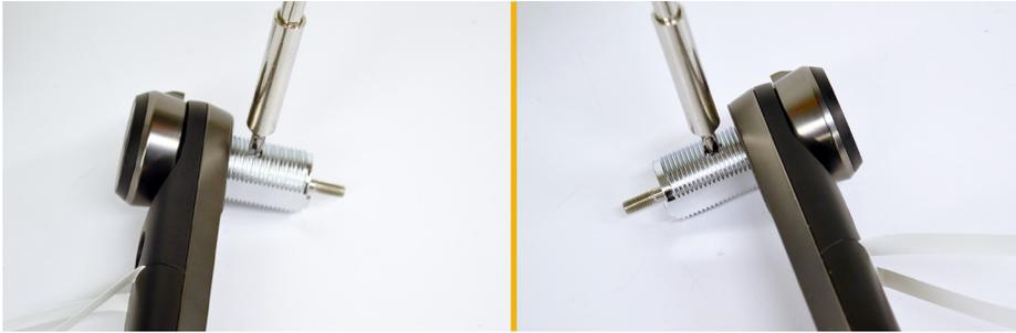
6 Insert and tighten the 2 small screws to secure the shaft adapter.
