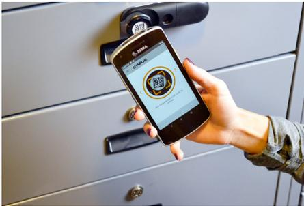
**30a Lock Activation Using Device Camera:** Open the InVue LIVE Access App on your smart device and toggle to the “Camera Scan” screen. Center the barcode in the viewfinder. Once confirmed by the App displaying “unlocked” and the LED flashing green.
