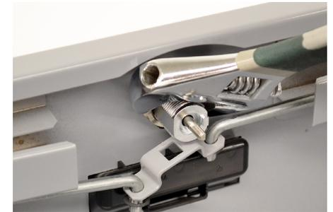
11 Use a wrench to tighten the nut.
