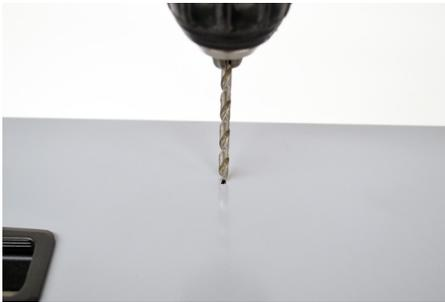
**3b** Drill a hole in the drawer face with a 3/16 inch (or 5mm) drill bit.
