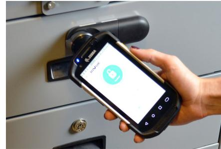
**27a** **Lock Activation Using NFC:** Open the InVue LIVE Access App on your smart device. Tap your device against the round panel on the lock. Once confirmed by the App displaying “unlocked” and the LED flashing green.
