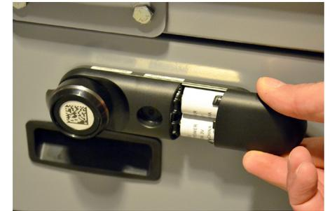
**32** Remove the battery panel from the lock.
