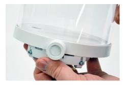
Center the clip beneath the IR lens so that the slots on the clip fit around the lens. Align the slots on the clip with the posts on the bottom of the Zips IoT Base.
