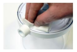
Use an alcohole wipe to clean the inside track on the bottom of the display plate near the IR lens. Allow it to dry completely.
