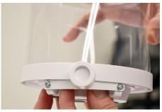
Press the clip against the bottom of the Zips IoT base for at least 10 seconds.
