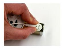
Place the sensor on the cleaned area on the shaver.
