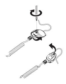
Press sensor firmly onto merchandise for 10 seconds. Wrap loop around merchandise. Tightly pull loop through sensor and tighten with T-20 bit.
