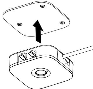
**4c** If routing the power cable through fixture, drill a 19mm hole minimum in fixture and direct the power cable straight down through the hole. Clean the surface of any dust or debris caused during drilling using the provided wipe and press alarm unit firmly against the surface for at least 10 seconds.
