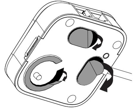
**4a** If mounting above the counter, route the power cable across the fixture surface to the power source. Press alarm unit firmly against the surface for at least 10 seconds.
