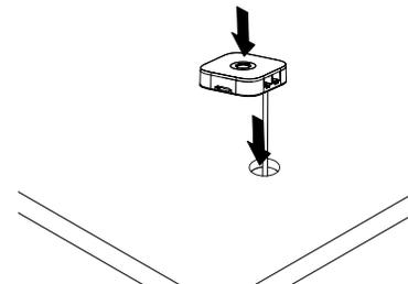
**5** For all mounting methods, be sure the plunger switch on the bottom of the alarm unit is engaged with the surface.
