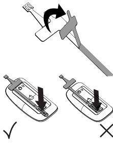
Grab sides of the cover on the sensor and pull back to expose the metal contacts.
