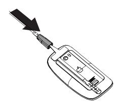
Plug the micro USB connector into a Zips! 2.0 alarm unit. The alarm unit will chirp.
