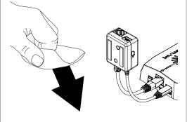
Peel the clear film from the adhesives on the bottom of the junction box.
