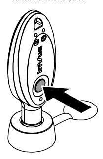
During an alarm event, the LED emitter will flash until deactivated. Place a charged and coded OneKEY onto the IR dot and press the button to deactivate.
