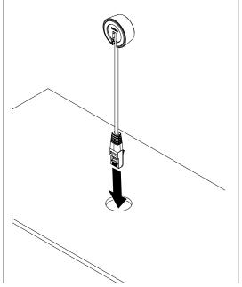
Plug the IR dot into the RJ45 port on the junction box.
