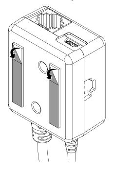
Place the junction box in the desired location and apply pressure for at least 10 seconds.
