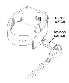
**Optional:** Insert secondary tear sensor (AC193/AC194) into sensor as shown. Confirm secondary sensor pads align with band sensor pins.
