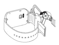
Note: Confirm secondary sensor, when installed (per Step 6) provides enough slack to open and close watch band. Watch charging pins should not be covered. Confirm watch will sit on cradle appropriately. Re-adjust band sensor accordingly.
