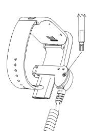
If using secondary tear sensor, clean back of watch with alcohol wipe provided. Let it dry completely. Peel film from adhesive.
