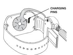
Place watch onto cradle (AC115-W) and firmly plug stand in Zips 2.0 alarm unit. The alarm unit will "chirp". Close alarm unit door.
