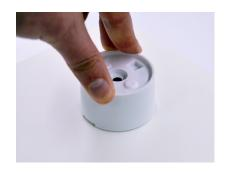
With the sensor port facing away from the customer position, place the unit onto the fixture and apply pressure for at least 10 seconds.
