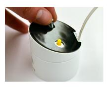
Insert the provided screw into the screw hole.
