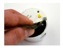
Peel the adhesive from the bottom of the alarm unit.
