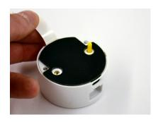
Pull the battery tab from the bottom of the Zips alarm unit.
