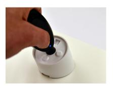
Use a charged and coded OneKEY to disarm the alarm unit when needed.
