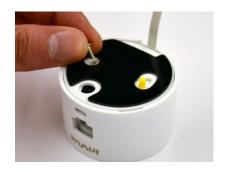
8 Insert the provided screw into the screw hole.
