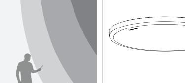
If using the LED Emitter, determine where it will be mounted. Use the provided alcohol wipe to clean the are where it will be mounted.
