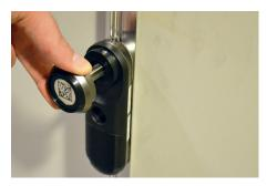
Once confirmed by the App displaying "unlocked" and the LED flashing green, you will have several seconds to pull the knob out and slide the door panel open. If the LED on the lock flashes red before the lock is opened, it will need to be unlocked again.
