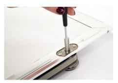
Insert and tighten the 4 smaller screws to secure the lock body to the door panel.
