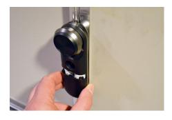
Slide the battery panel back into place.
