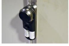
Replace the old batteries with new CR123A non-rechargeable lithium batteries.
