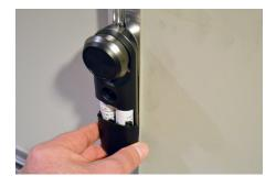
Remove the battery panel from the lock.
